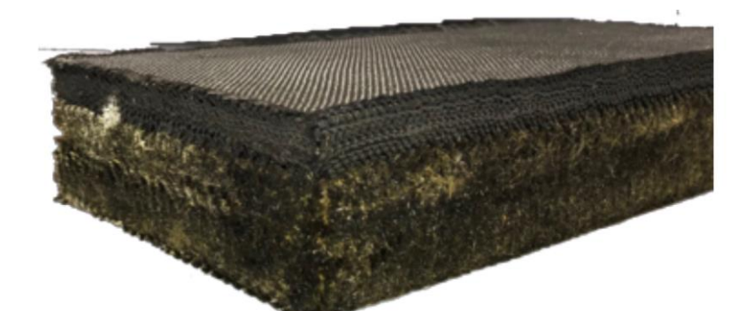
Fig 11. HEEET 3D Woven Preform. Credit: NASA
