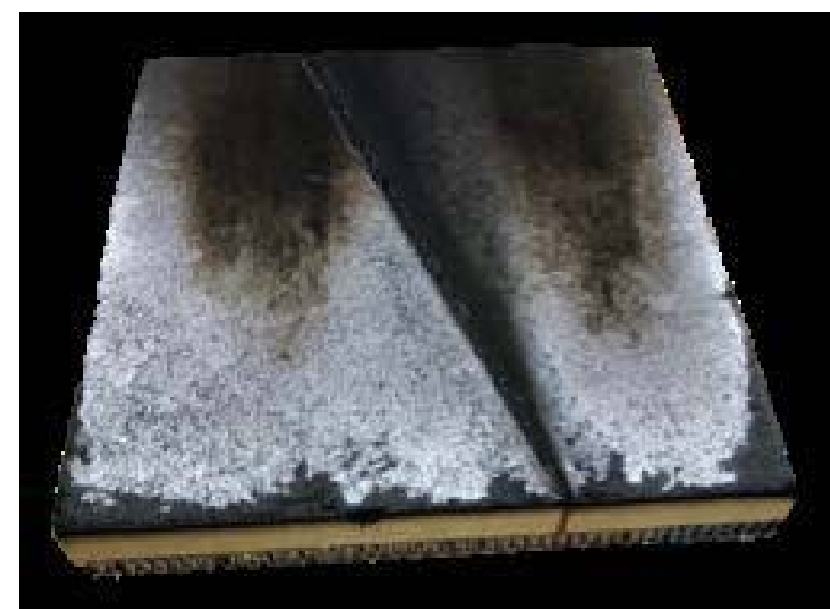
(b) A section of tested PICA TPS with NuSil surface coating [2].
