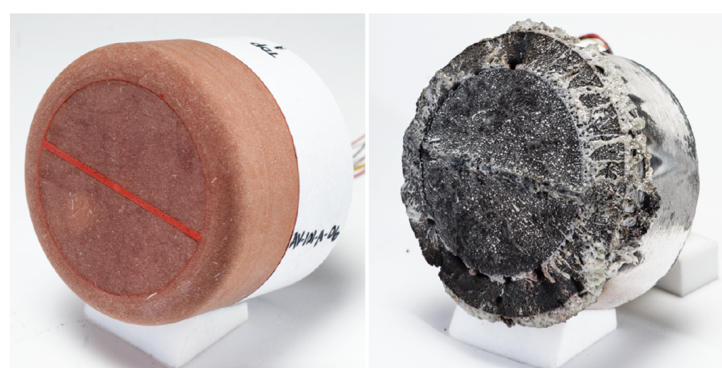
(a) Avcoat specimen showing formations from molten silica layers, before (left) and after (right) testing [1].
