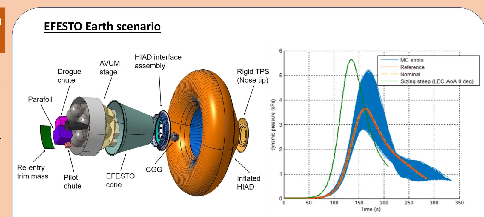
System configuration and sizing dynamic pressure profile
